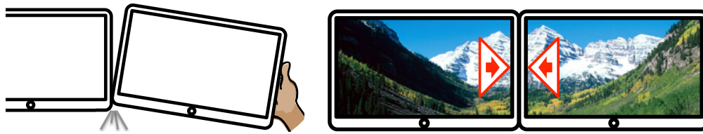
Fig. 8. An illustration of “Synchronous Gestures” [Hinckley 2003]: (Left) A user connects two devices by bumping one device into another one. (Right) “Dynamic Display Tiling”, an application based on Synchronous Gestures. A user annexes the displays of two tablets, allowing a panoramic image to span both displays.
