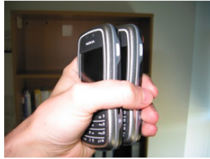
Fig. 7. “Shake Well Before Use” [Mayrhofer and Gellersen 2007b; 2009]: A user holds two mobile devices in one hand and shakes them rapidly for several seconds to establish an association.
