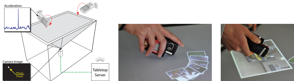
Fig. 9. “PhoneTouch” [Schmidt et al. 2010]: (Left) An illustration showing how the system detects phone tapping events. (Centre) A user drops a collection of photos on a surface. (Right) A user picks up a photo by tapping on it. (Source: Dominik Schmidt)
