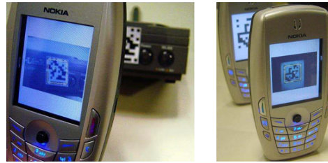
Fig. 3. Examples of “Seeing-Is-Believing” (SiB) [McCune et al. 2005; 2009]. A phone running SiB scans the barcode of a target device to capture its cryptographic information. (Left) Static visual barcode. (Right) Dynamic visual barcode. (Source: Jonathan McCune)
