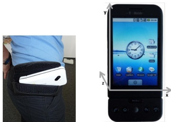
Figure 2: Phone attached to the subject and the three axes in which acceleration is measured [21].
