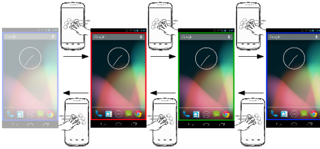
Figure 2: The Swipe switching mechanism allows to switch between security zones in a circular manner. This is done with a horizontal (left or right) three finger swipe.
