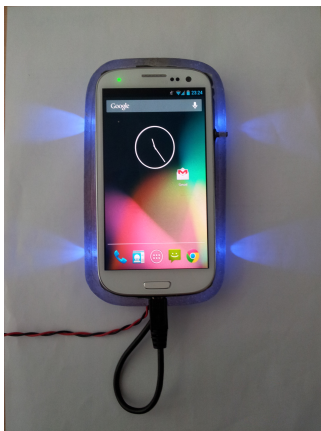
Figure 5: The custom cast resin housing including LEDs for zone visualization at the example of the Managed zone.
