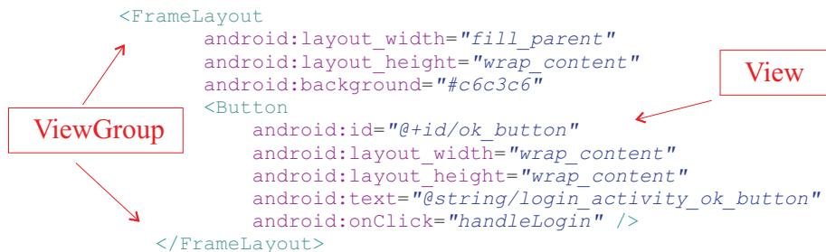
**Fig. 1.** XML definition of a Button (View) which is embedded in a layout (ViewGroup)
